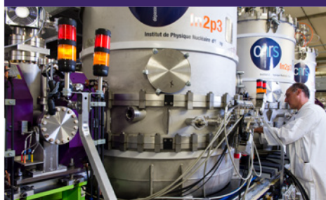
Cryogenic chambers enclosing the accelerating cavities of the SPIRAL2 superconducting accelerator.
